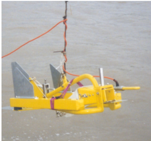
Fig. 69: The Helley Smith bed load sediment transport meter (BfG, 2008)
