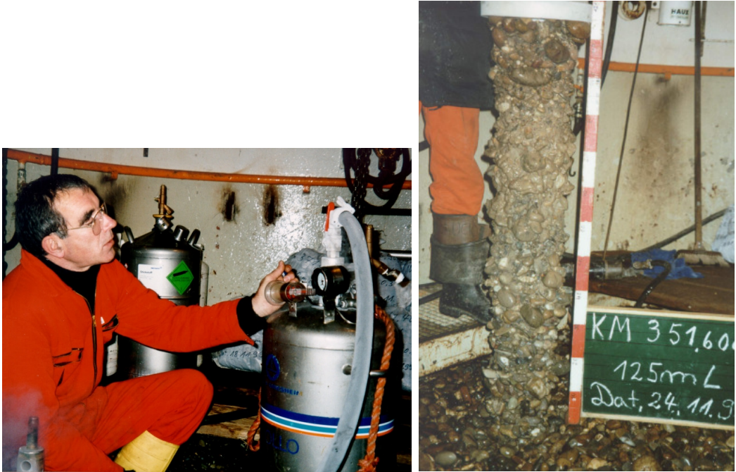
Fig. 64: Freeze-coring in the diving-bell (BfG, 2008)
