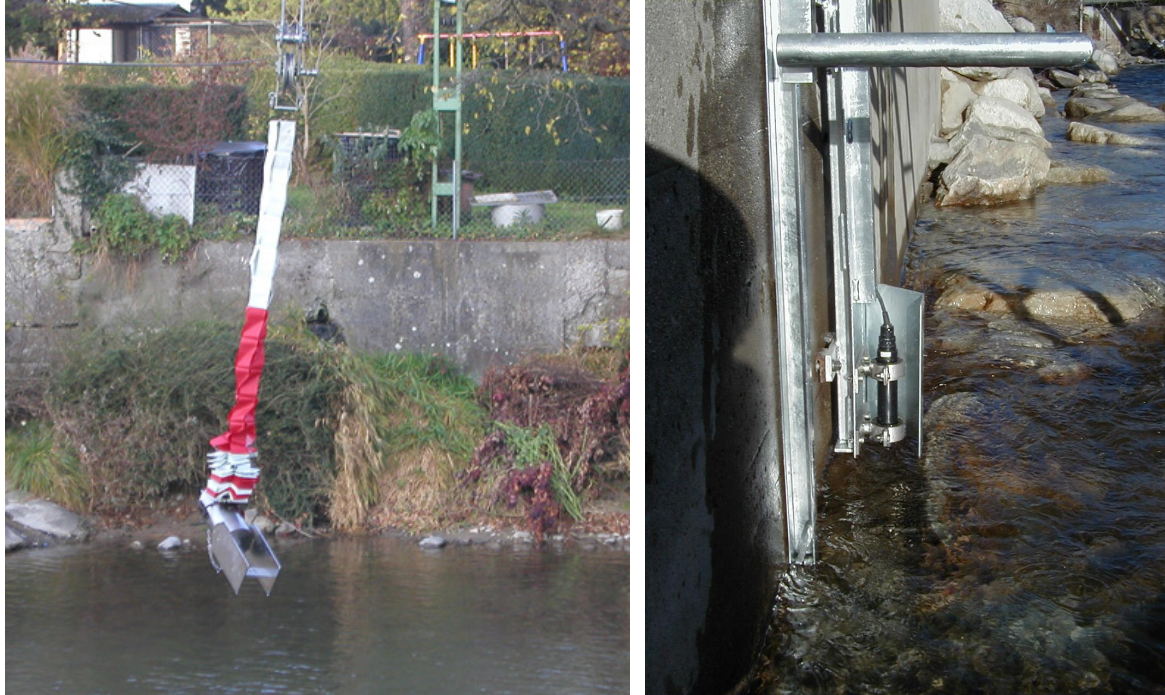
Fig. 60: Suspended sediment sampling device (left); Turbidity sensor (right) (Grasso, et al. 2007)
