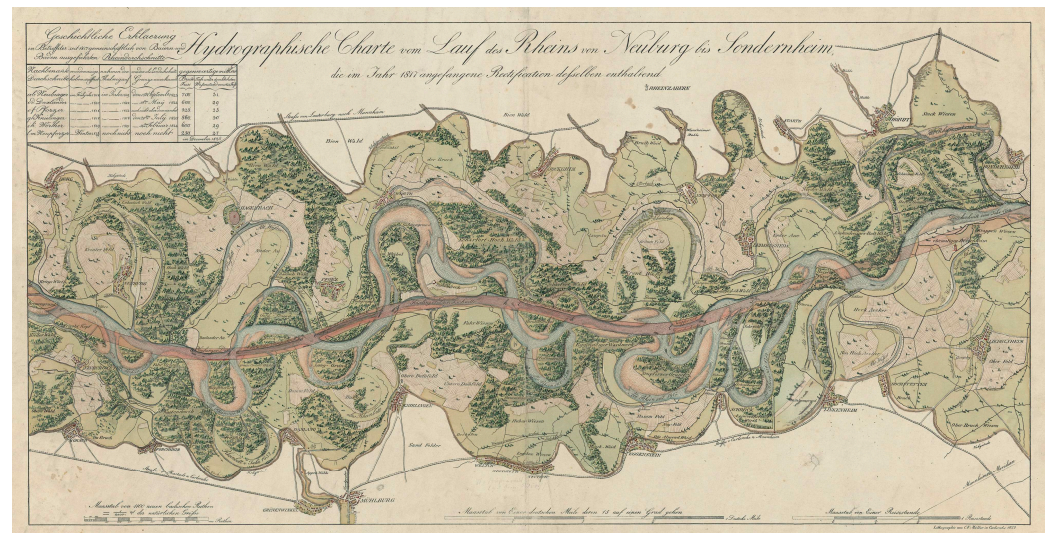
Figure 5. The Rhine River system between Neuburg (rkm 355) and Sondernheim (rkm 380) indicating river channelization in 1817 (Source: Generallandesarchiv Karlsruhe, H Rheinstrom 72, http://www.landesarchiv-bw.de/plink/?f=4-1736483-1 , accessed on 26 February 2024).
