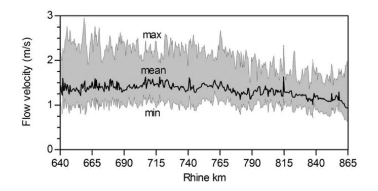
**Fig. 2.** Longitudinal velocity profile of the lower Rhine Embayment (SOBEK model computation, period 1993–2010).
