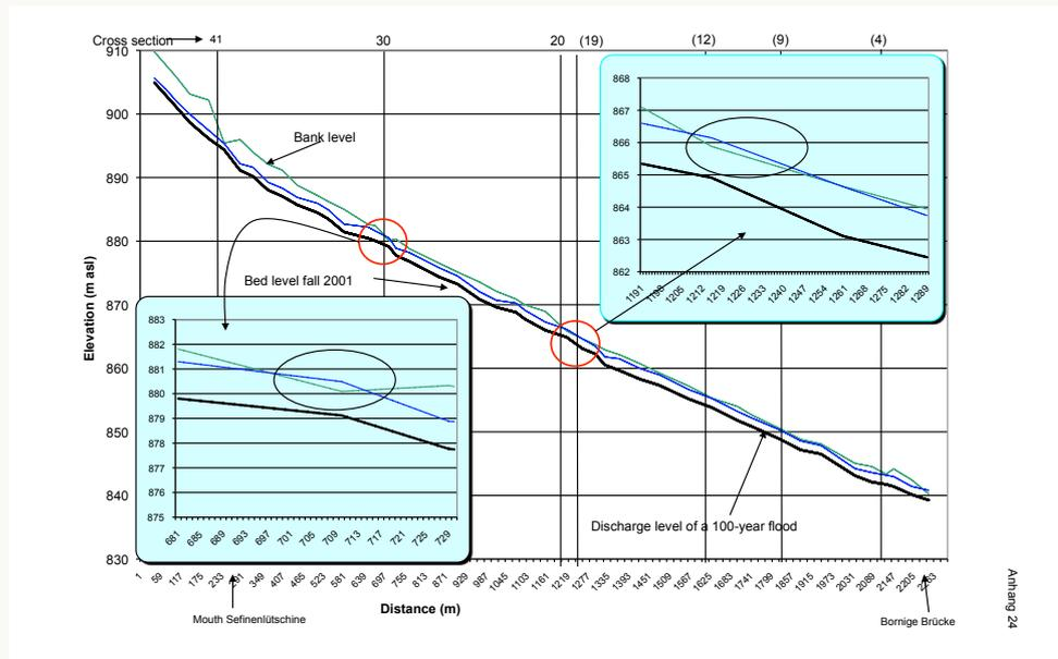
Figure 2.24 Bed- and water level in the case of an event of 100 year recurrence interval indicating potential places of river outbursts
