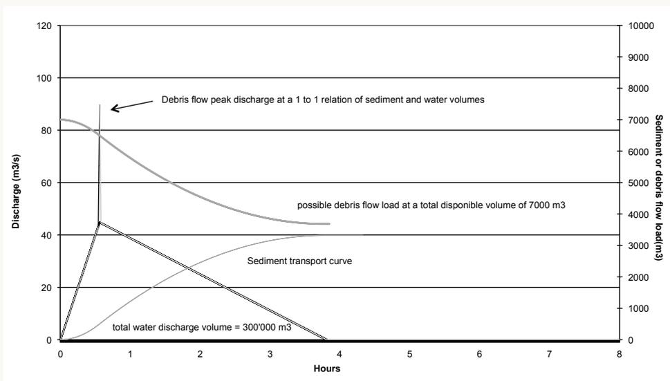
Figure 2.26 Debris flow load and peak discharge assessment for a debris flow in the Grönbach, Bernese Oberland
