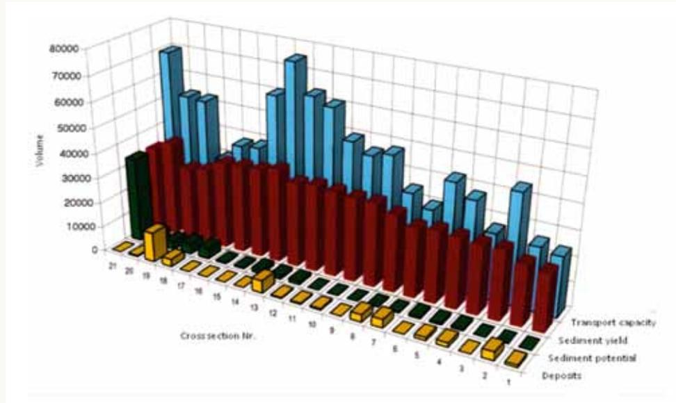
Figure 2.21 Sediment transport during a large event in the Guppenruns, canton of Glarus
