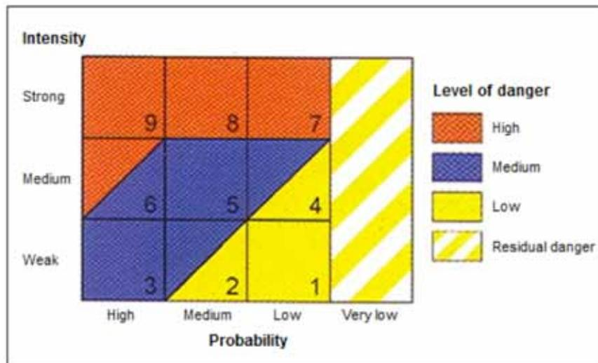
Figure 1.6 The 4 hazard categories used in Switzerland with consequences for building and zoning regulations (Swiss Federal Office for the Environment, CH-3003 Berne)
