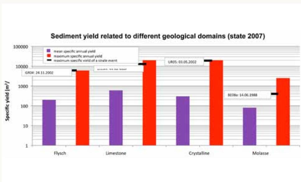
Figure 1.8 Analysis of the observation of total bed load gained by sediment retention basins, structured according to geological formations (blue = mean specific annual volume, red = maximum specific annual volume, black line=maximum specific volume of a single event). (A. Grasso, Swiss Federal Office for the Environment, CH-3003 Berne)
