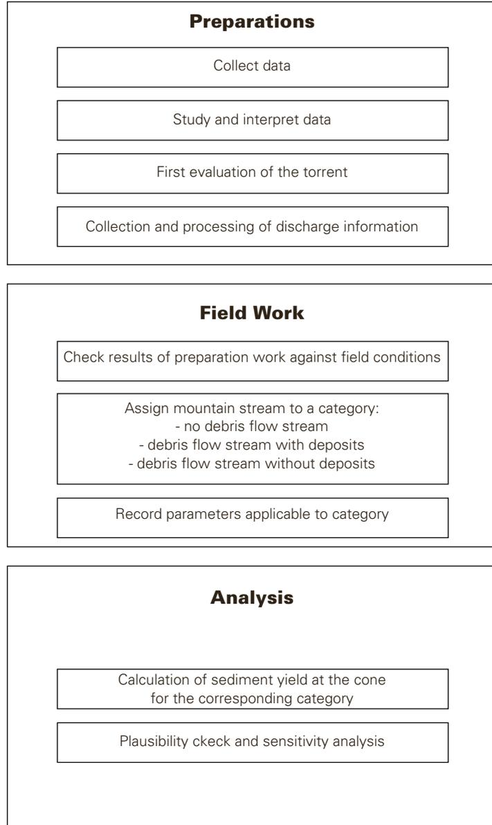
Figure 2.9 Overview of the steps required for the assessment of sediment yield
