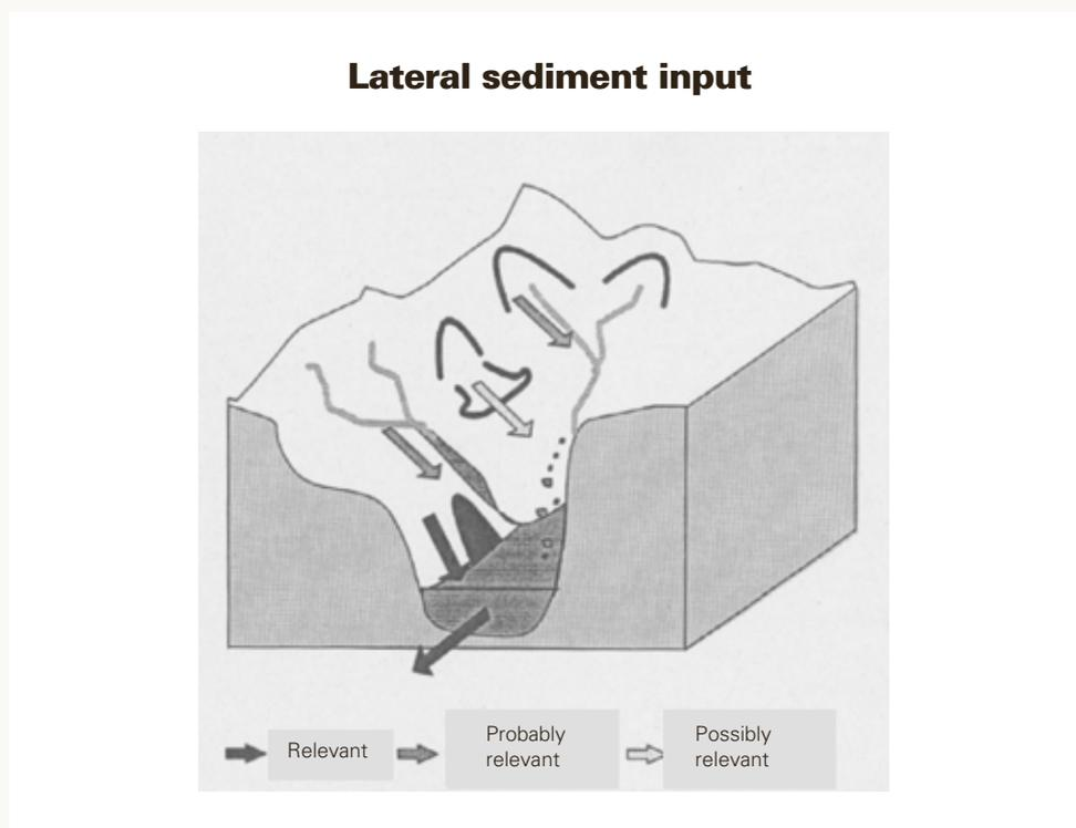
Figure 2.7 Relevance of sediment sources
