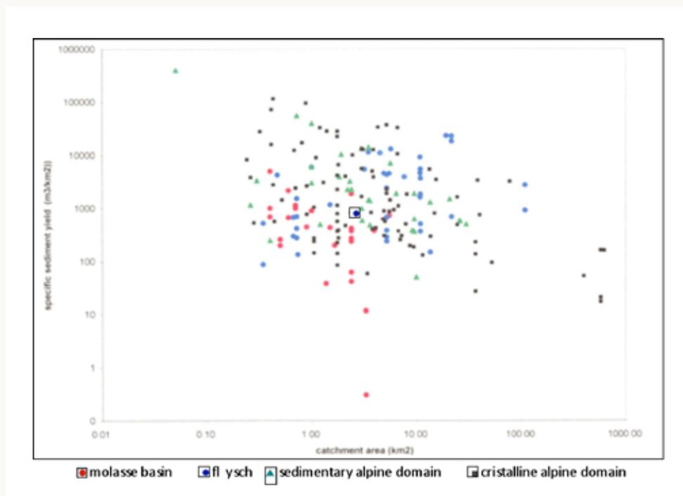
Figure 2.10 Specific sediment yields in 4 geological categories of past events in Switzerland
